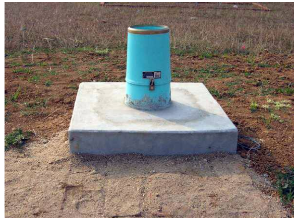
Fig 1.2 Ground surface installed Symons rain gauge
